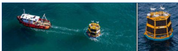
(Top) RPS LiDAR buoy being towed to site and deployed on its mooring. (Bottom) Wind speed overlay plot measured during the trial by the LiDAR buoy (blue) and the reference LiDAR (red) for the duration of the deployment.
