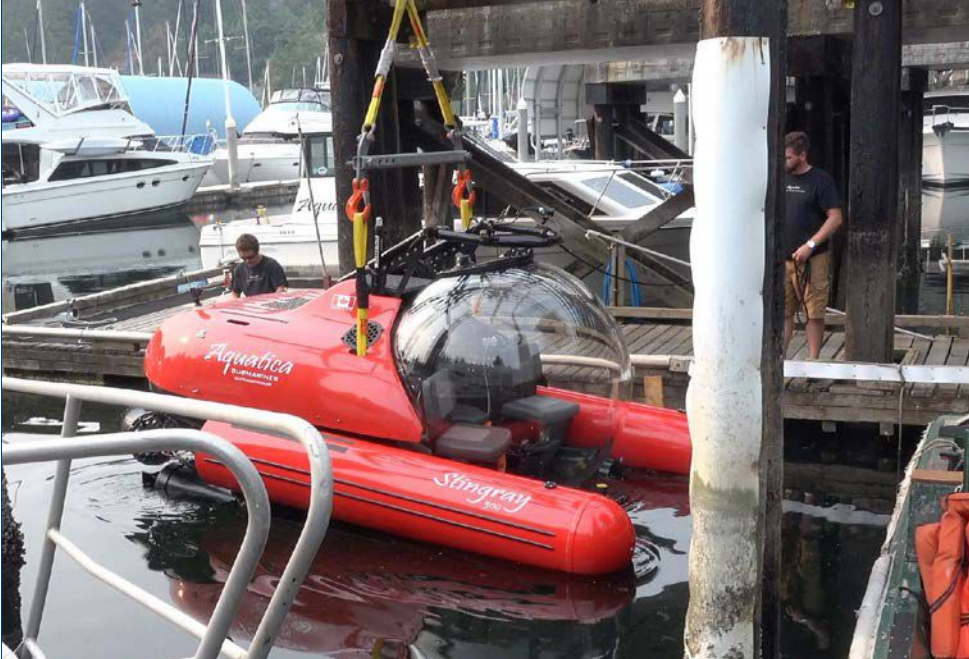
(Top) The prototype Stingray 500 three-man submersible being deployed by crane at the marina launch site close to the dive site. (Bottom) A juvenile male sixgill shark estimated at 2.0 m tl, adjacent to ballast chamber of Aquatica manned submersible (diameter of chamber 60 cm for scale). Sharks were highly attracted to metal and electrical elements of the submersible.
