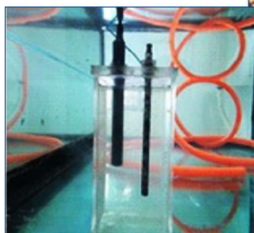
Lab testing of single-cell prototype underwater battery.
