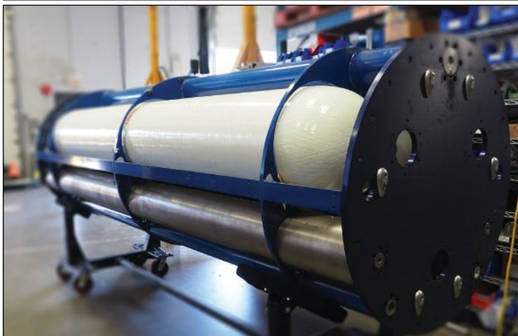
(Top) Solus-LR base UUV configuration in Cellula's test tank for early testing of controls and telemetry. (Bottom) Solus-LR fuel cell module, with hydrogen, oxygen and wastewater tanks shown.
