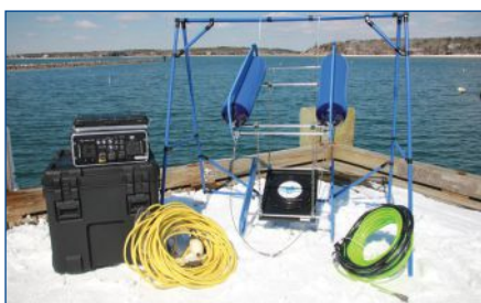
Complete Bubble Gun standard single-source system shown with the single-channel hydrophone and system shipping case.
