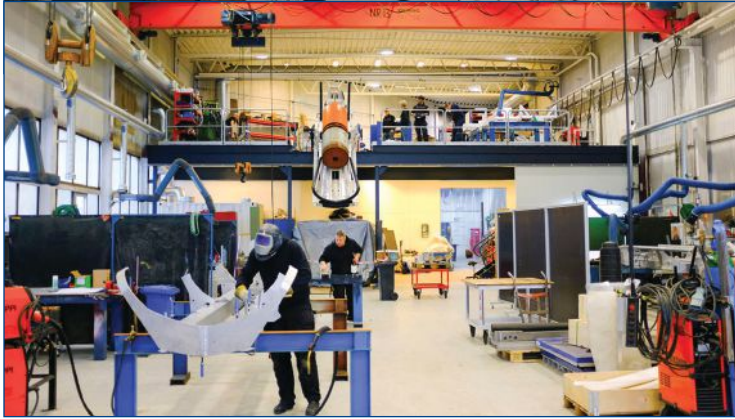
(Top) Henriksen Marine Division workshop in Tønsberg. (Bottom) An AUV launch and recovery system under construction in the Henriksen Marine Division workshop.
