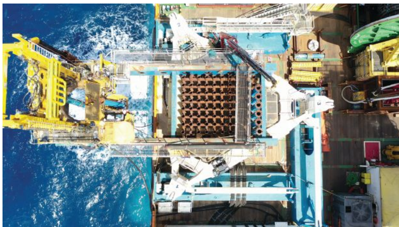
(Clockwise from top left) The drilling operation in the Caribbean Sea, off the coast of St. Croix, U.S. Virgin Islands. The LDD drill rig was cantilevered off the Barge Master motion-compensated platform. The drilling location had a rough swell, and the drill combination worked in weather conditions up to Hs 2.5 m. Top view of the drill rig on the motion-compensated platform.
