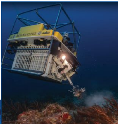
(Top) ReefSweeper about to retract its spear and draw a lionfish into the vehicle. (Bottom) A lionfish has just been speared by ReefSweeper.
