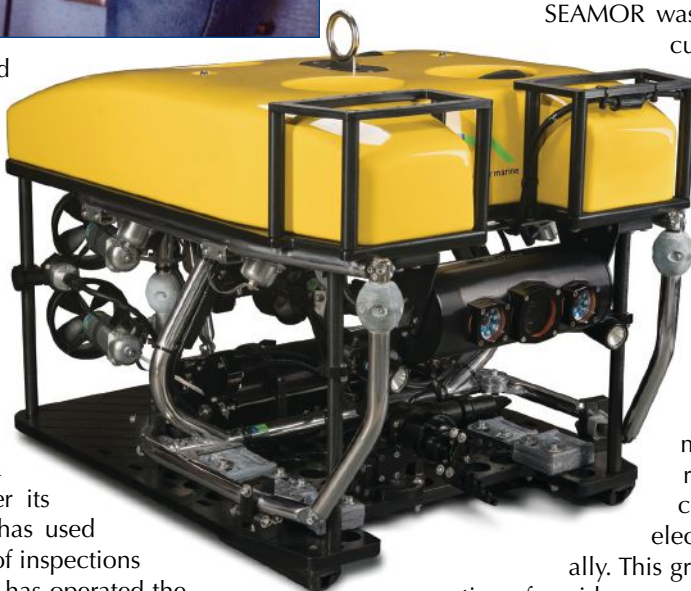
Legendary engineer Al Robinson and entrepreneur Terry Knight were responsible for SEAMOR Marine's first prototype in 1989. (Below) The Mako ROV is SEAMOR's largest ROV. It can support a payload of up to 22.5 kg and work at depths up to 600 m.
