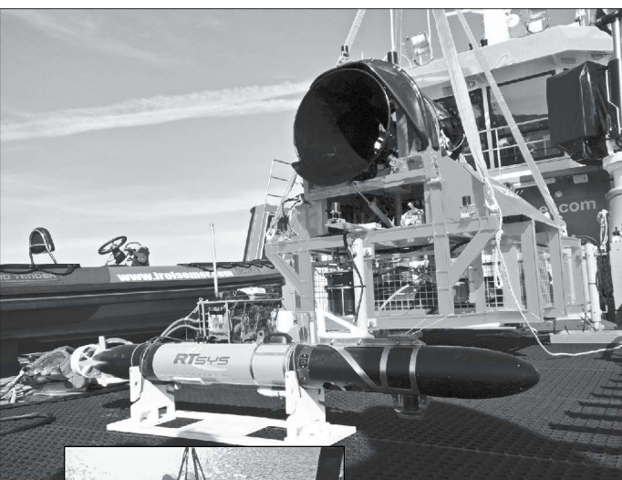
The Naval Group docking station and RTsys Comet AUV.
