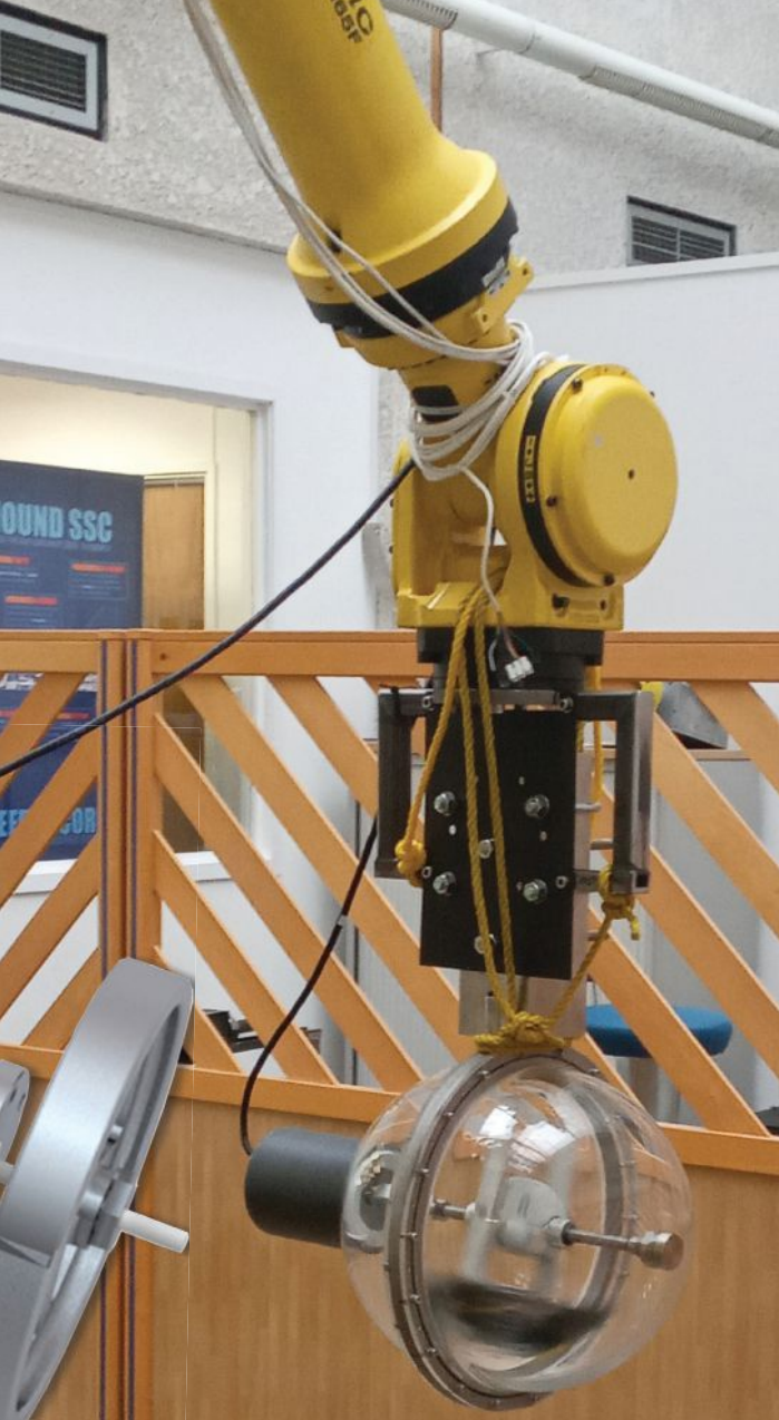
(Far left) The WITT system being tested in our Fanuc in-house robotic arm, demonstrating power from VIV. (Above) Small WITT unit, proving we can harvest 6° of motion. (Top right) WITT larger-scale system. (Bottom right) Large WITT unit being tested at Southampton University.
