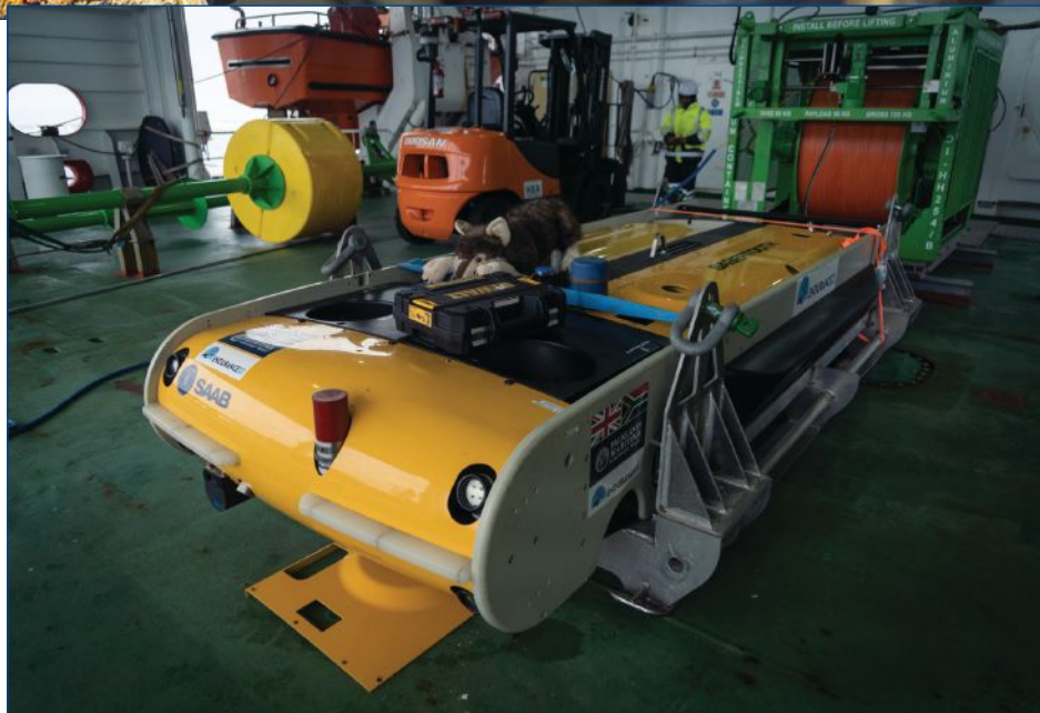
(Top) Extrusion of low-density outer jacket. (Bottom) LIN-DEN-SPE-7098 attached to Saab Sabertooth ROV. (Credit: Falklands Maritime Heritage Trust)
