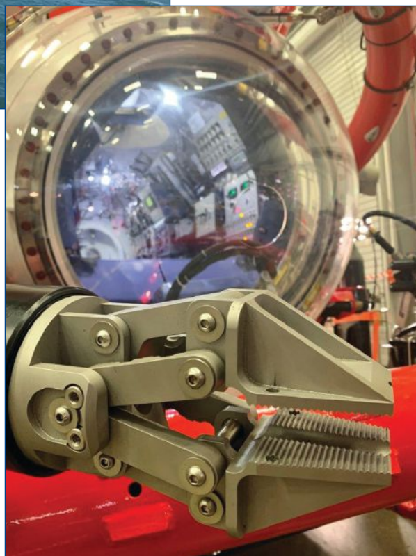
FET's ROV during sea trials in Vietnam. (Below right) LR11 command module and manipulator claw.
