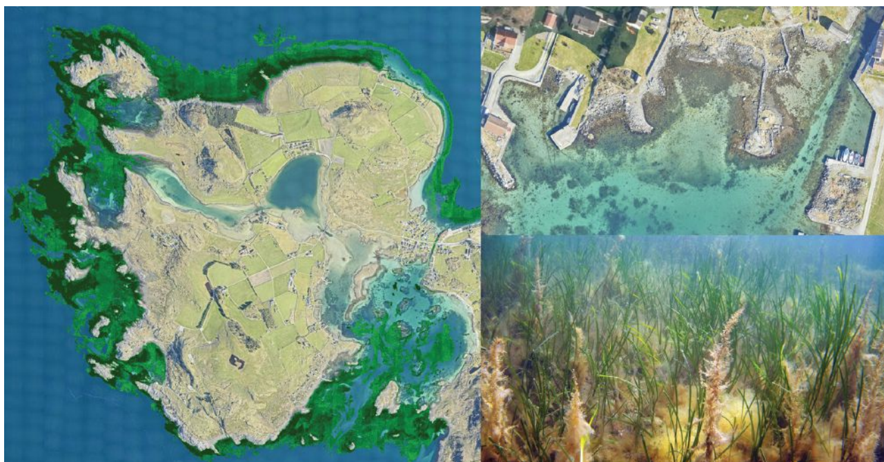
Mapping marine vegetation using a sensor fusion of ALB and RGB/hyperspectral imagery.
