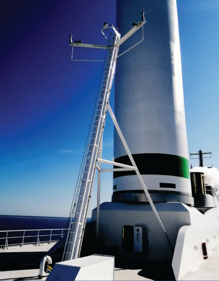
(Top) A closeup of the Rotor Sail and Vaisala's WMT700 wind sensor. (Credit: Norsepower) (Bottom) MARIN teamed up with Econowind and utilized Vaisala's WindCube Scan technology to measure wind conditions on a vessel equipped with two of Econowind's VentoFoil, which are aerodynamic, wing-shaped elements integrated with smart suction to create a high propelling force.
