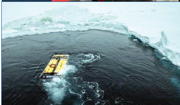
Saab Sabertooth, a deepwater hovering hybrid AUV/ROV, was deployed to the depths of the Weddell Sea in Antarctica, housing Covelya Group technology, as part of the expedition that discovered Shackleton's Endurance. (Credit: Falkland Maritime Heritage Trust)
