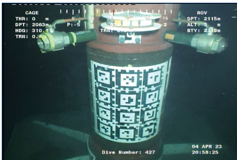
(Top) Target adhered to a subsea structure. (Bottom) HaloCAM mounted to an ROV.
