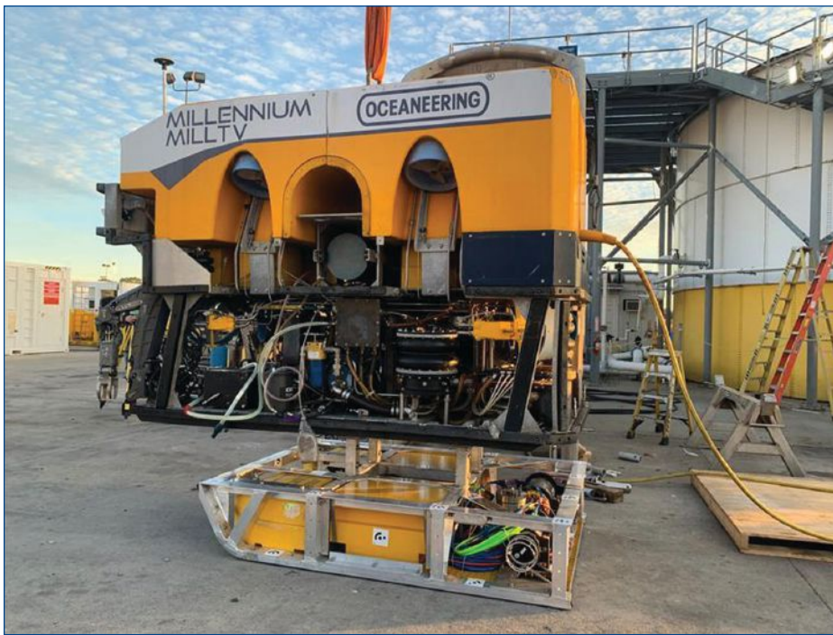
(Top) WROV Perception XL dynamic laser scanning skid with technology from EIVA, Sonardyne and Voyis. (Bottom) EIVA's VSLAM software with Voyis's Discovery stereo data acquisition.
