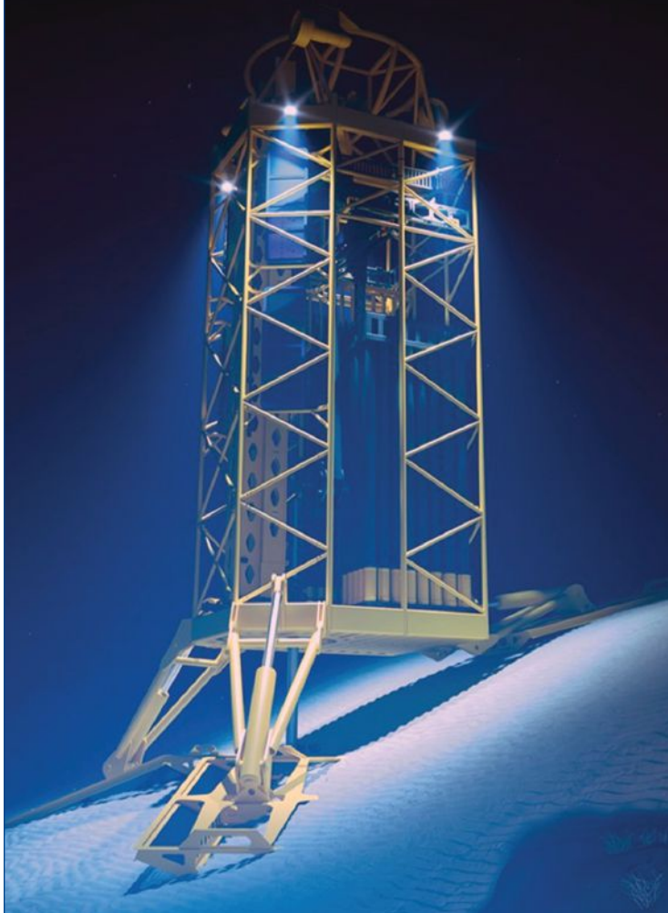
Rendering of the Fugro Blue Dragon next-generation seafloor drill, capable of operating at steep slopes in deep waters up to 1,500 m.
