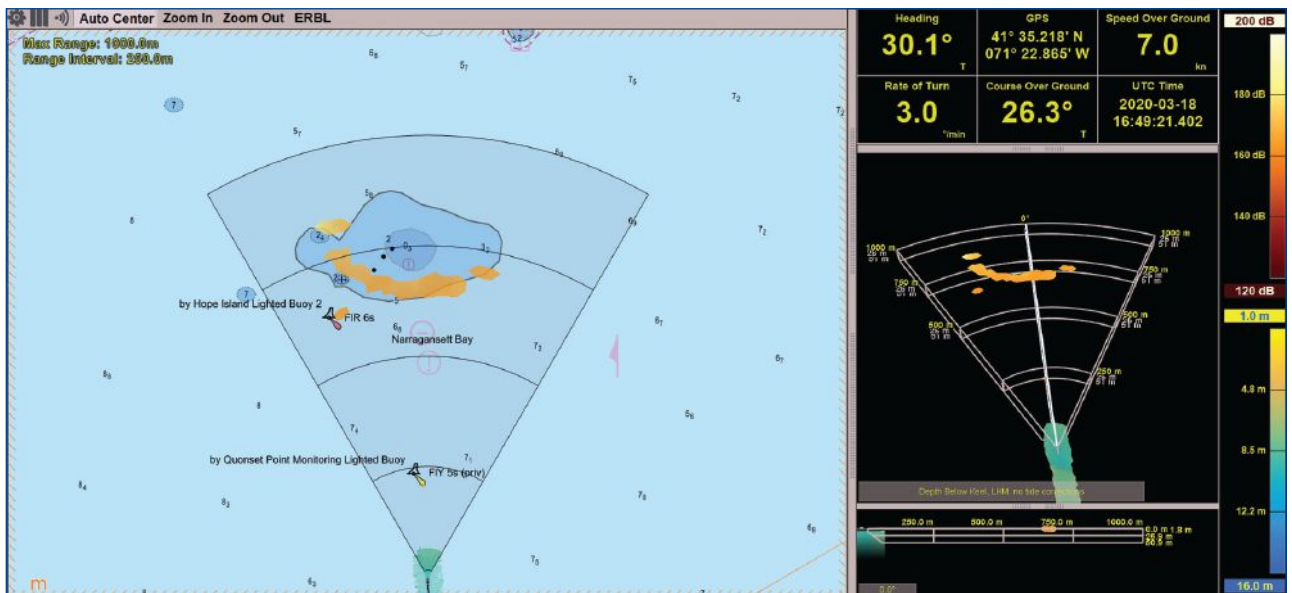
(Top) Screenshot from SonaSoft using an Argos 1000 to approach a submerged hazard (Boiler Awash in Narragansett Bay, Rhode Island). If a vessel were navigating around this obstacle purely on the chart and the location information from its GPS, it would be vulnerable to GPS spoofing and could be misled into danger by a bad actor. (Bottom) Screenshot of SonaSoft 3D Viewer demonstrating a steep change in depth.
