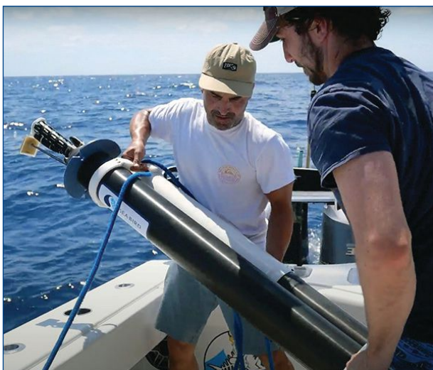
(From left) Michael Zedelmaier and Miles Mallinger, both of Seatrec, deploy a float with one of the company's SL1 power modules in the Gulf of Mexico before the 2022 hurricane season to collect data that could improve hurricane predictions. (Credit: Seatrec Inc.)
