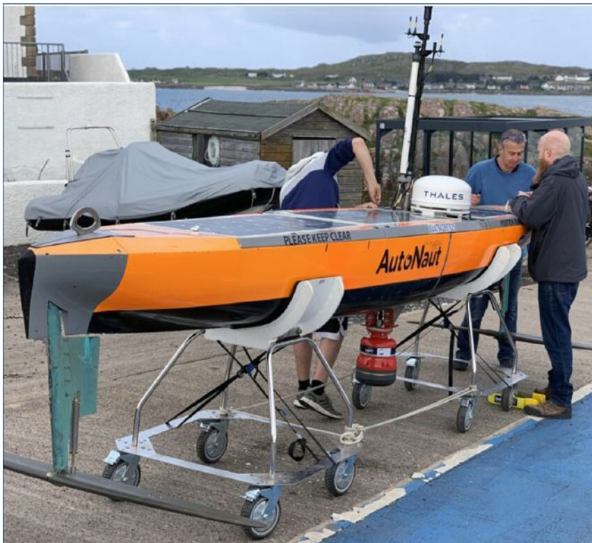
(Top) A Sonardyne Fetch BPR was moored at 1,800-m depth in the Rockall Trough. (Credit: Ben Moat, U.K. National Oceanography Centre) (Bottom) AutoNaut being prepared for launch. A Sonardyne HPT 3000 acoustic transceiver for through-water communication is mounted centrally, below the hull. The Thales VesseLINK 700/Iridium Certus satellite enabled scientists ashore to control the transceiver remotely. (Credit: Scottish Association for Marine Science, SAMS)
