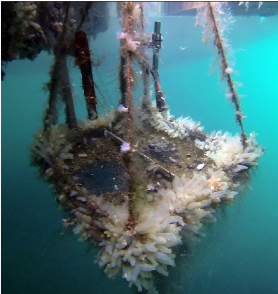
The contrast between the macrofouling that has developed and the clear areas illuminated by UV-C technology is visibly evident.
