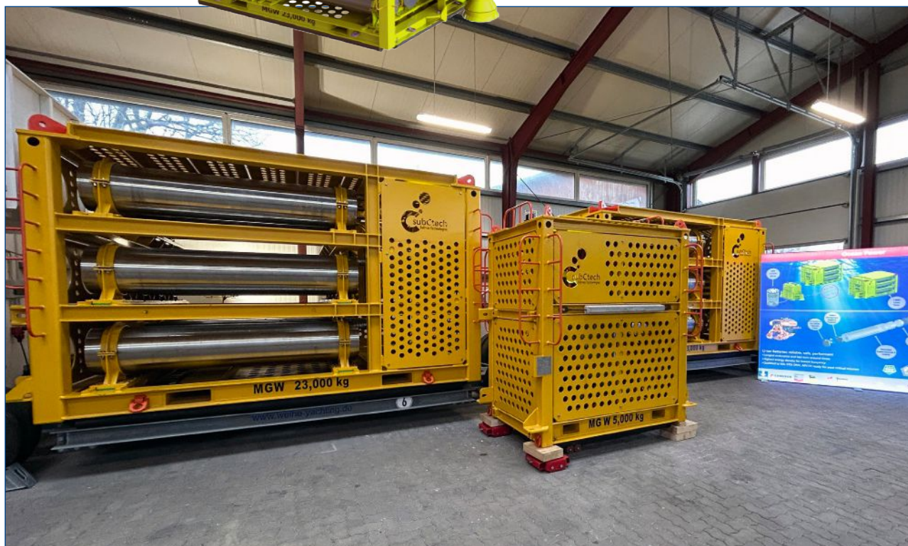
An illustration of SubCtech's 2-MWh energy storage skid, depicting two BSS and one power skid/converter. (Below) 2-MWh energy storage skid ready for shipment after factory acceptance test.
